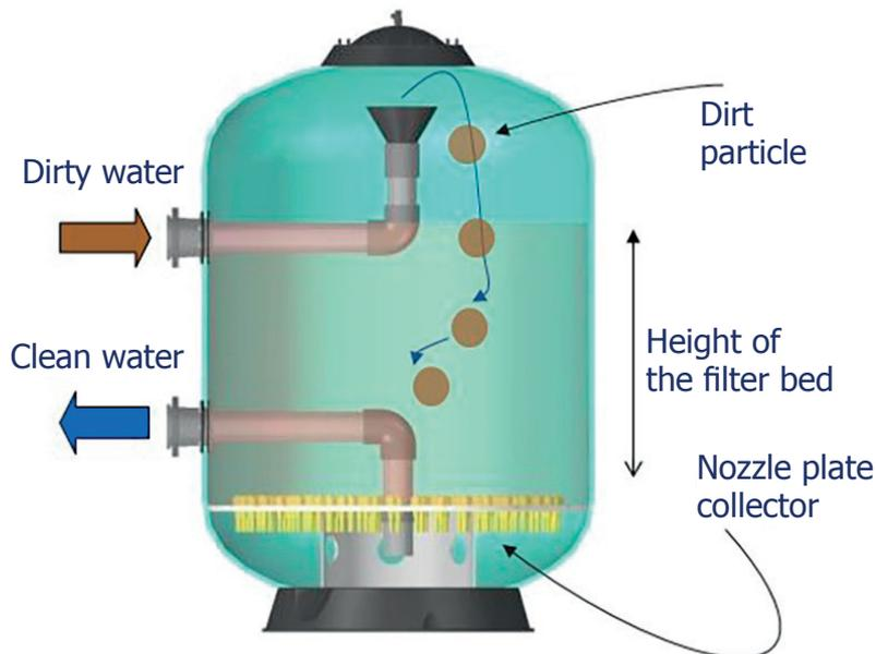
Image: Pathway of a dirt particle inside the filter
