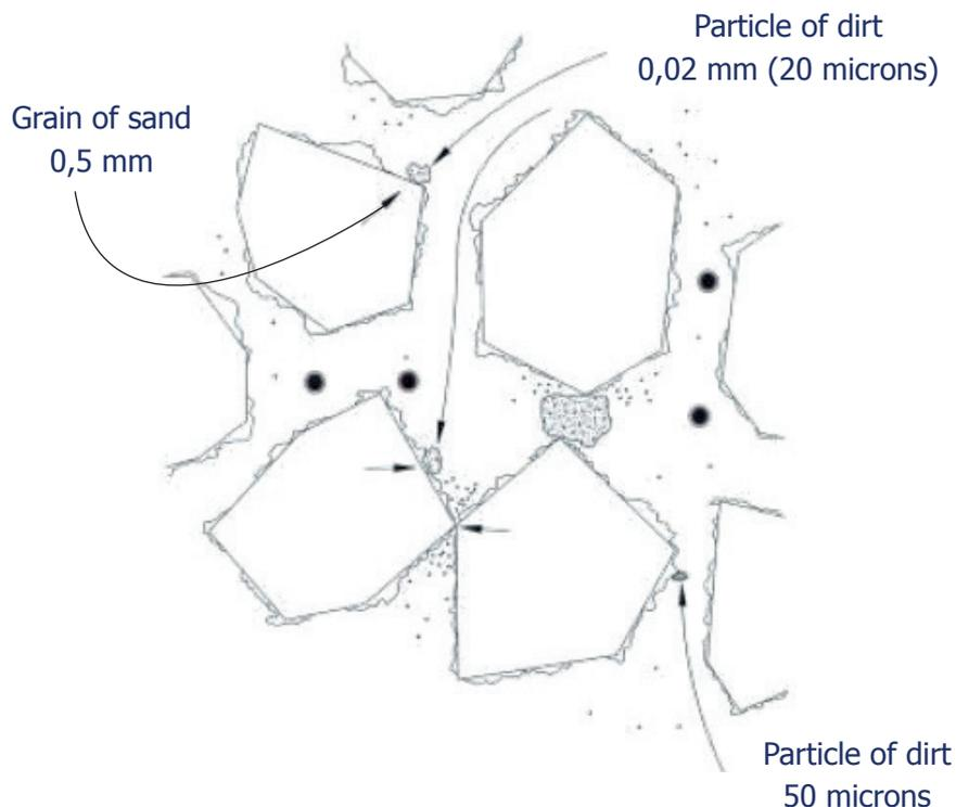
Image: Filtration mechanism in a granule media
